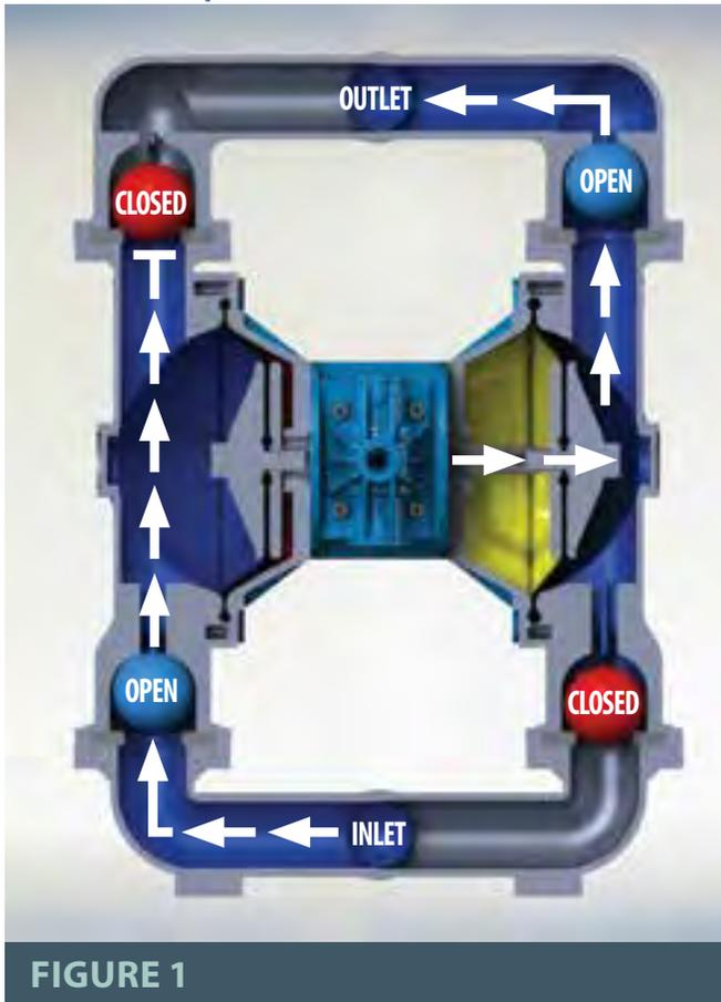
As the common shaft located in the center section moves to the right, the diaphragm in the left chamber moves towards the center section. This movement creates a vacuum on the liquid side of the left diaphragm, lifting the lower ball check valve, allowing liquid to flow through the suction manifold into the liquid chamber. At the same time, any fluid in the right chamber is discharged.
