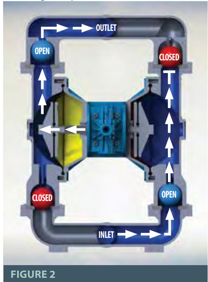
The air distribution system senses that the diaphragm in the right chamber reaches the end of its discharge stroke and causes the common shaft to shift. This moves the diaphragm to the left pressurizing the liquid, lifting the upper ball check valve, allowing fluid to flow through the discharge manifold and out of the pump.
